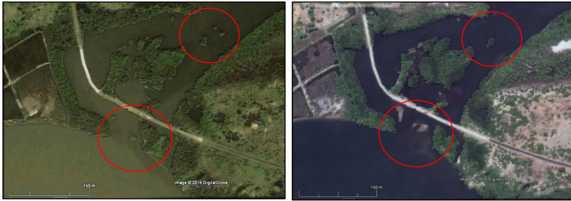
Figure 6 Google Earth remote sensed imagery over Nasivanthivu bridge and mangrove cover changes between 2004 (left) and 2016 (right). The red circles indicate erosion along the bottommost lagoon (Valaichchenai Lagoon) shoreline and 2 small islands have disappeared in the upper left corner. The patches just above the road have experienced increased mangrove cover.
