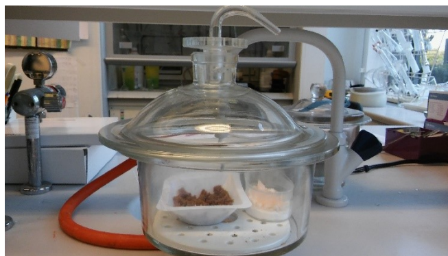
Figure 2.5: SE spruce sample drying in a vacuum desiccator. The sample is to the left and the phosphorous pentoxide drying agent is to the right. The silica gel is in the chamber below.
