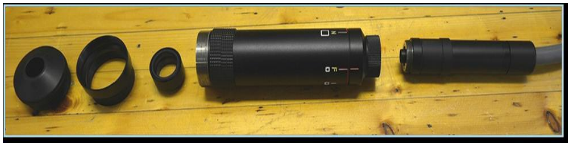
Figure 4. Setting of the video microscope: from right to left (in order of assembling): CVM video probe head from Micro Viper portable computer; Allen zoom lens, 20x – 120x basic lens; contact head adaptor; 60x-420x contact head.
