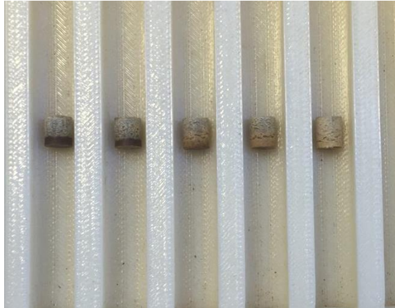
Photo1. Lower side of the pellets presents the position of the compacts based on the blank side of the die, in single-pellet rig. These sides of all pellets showed darker color than upper sides (on the side of compressing rod in single pellet method).
