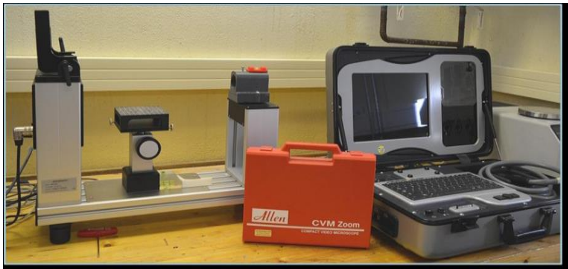
Figure 1. Equipment used for the evaluation of UPS swelling (left – Krüss tensiometer, center –Allen zoom compact video microscope lenses, right – Micro Viper portable computer.
