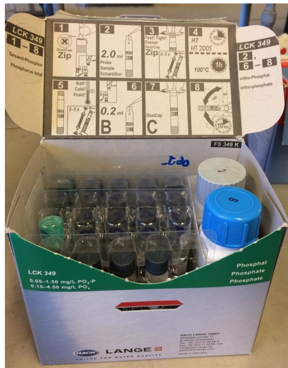
Fig. 3.7: Kit LCK 349 with work steps.
