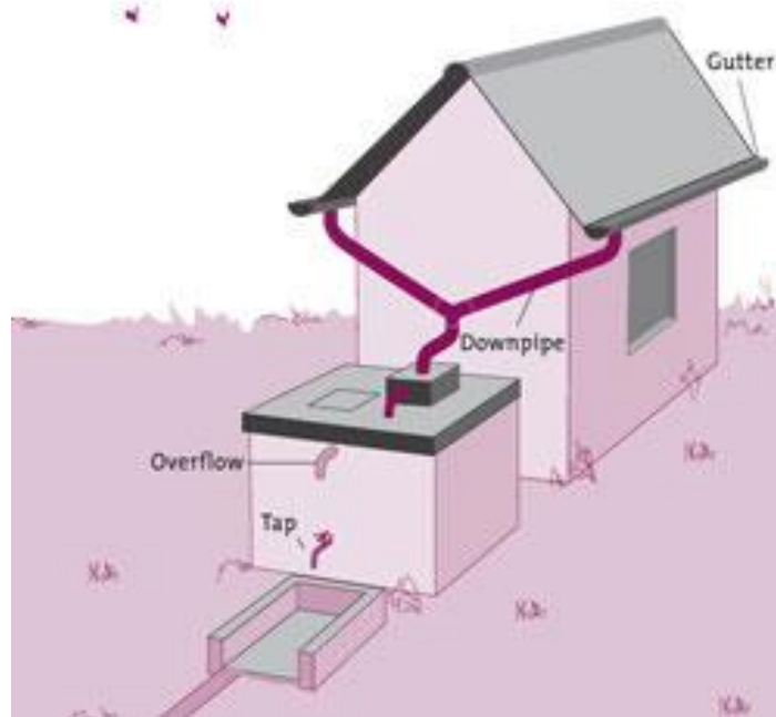
Fig. 1 Rooftop rainwater collection system (Smet 2003)
