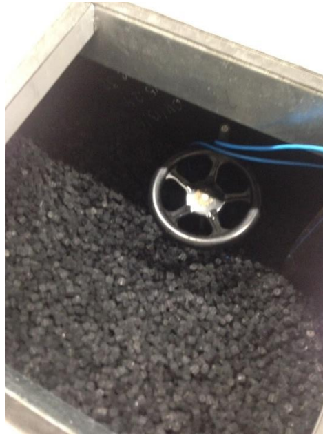
Figure 3.8.3: Clogged SBR with biochips (Levik, 2017b).
