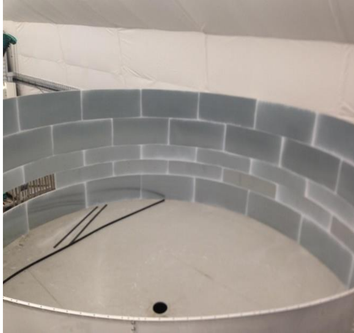
Figure 3.4.2: Tank without water showing central drainage (Levik, K., 2017b)
