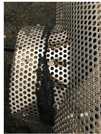
Figure 6.6.1: MBBR and SBR (yellow) Figure 6.6.2: Construction failure in grating
