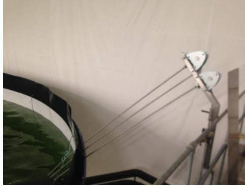
Figure 3.7.3.1: Manual operating pulley system for dead fish collection (Levik, K., 2017b)
