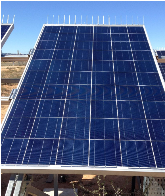
Figure 3.2: Left: The Rene Sola polycrystalline silicon module. Right (Armand du Plessis, by permission): The First Solar cadmium telluride module.
