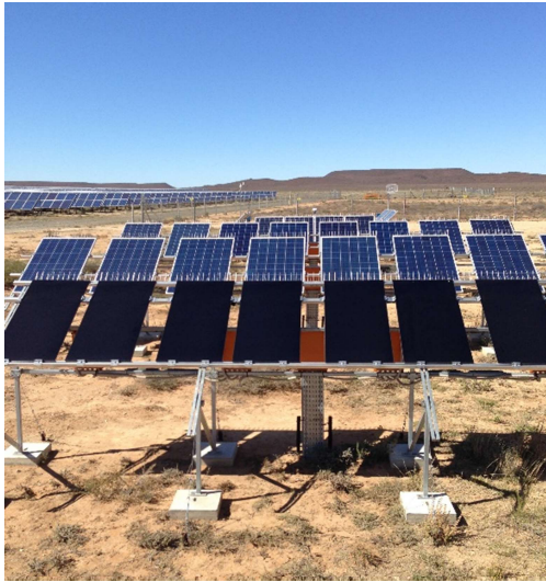
Figure 3.1: The set up and numbering of the three different types of modules on the test site. Behind the three rows of modules used in the analysis is a row with modules charging batteries that provide power to the measuring equipment. The weather station is located behind the fourth row.
