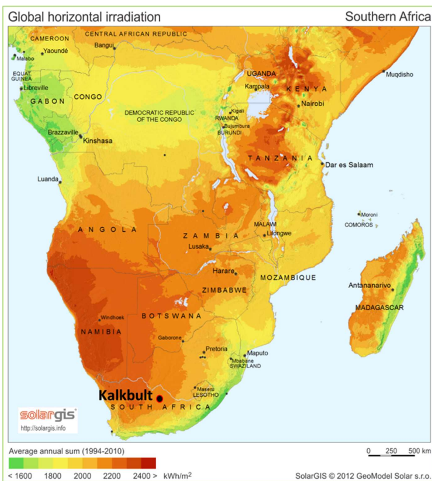
Figure 3.3: The average annual insolation in the southern part of Africa. The approximately location of Kalkbult is marked with a black dot. From GHI Solar Map © 2016 Solargis. (Solargis 2016)
