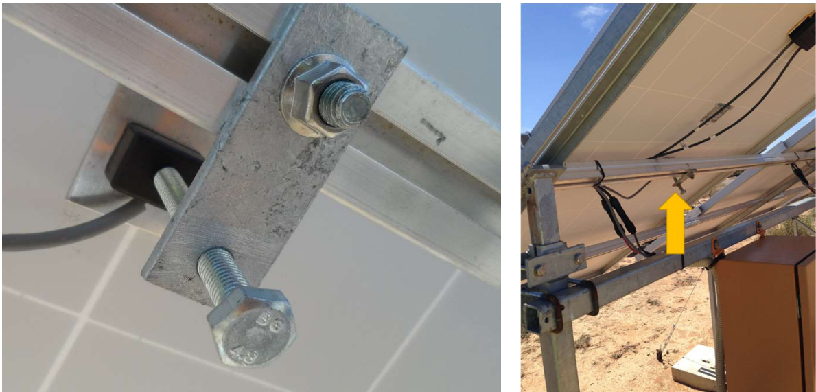
Figure 3.11: The ADT7310 temperature sensor, mounted at the back side of the module. Left (Armand Du Plessis, by permission): mounting of temperature sensor. Right: position of the sensor on the module.
