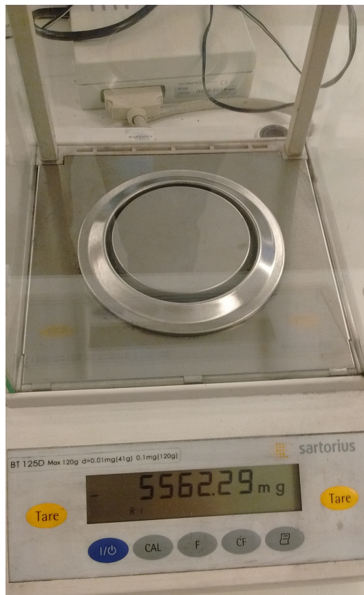
(b) Weight scale. Has an uncertainty of \pm 0.01 mg.
