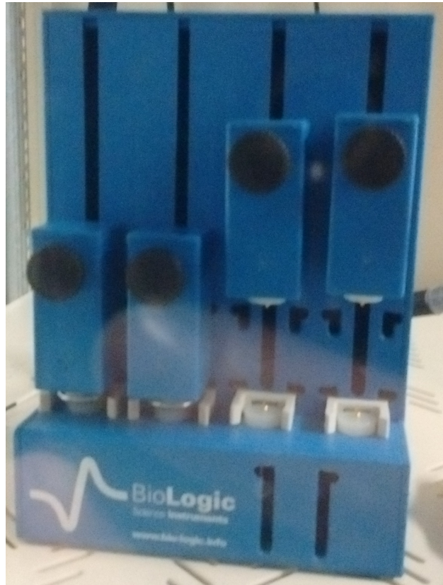
Figure 3.6: The Bio-Logic Science Instruments' product used for cycling cell EA. The main purpose was to perform an EIS study on the cell.
