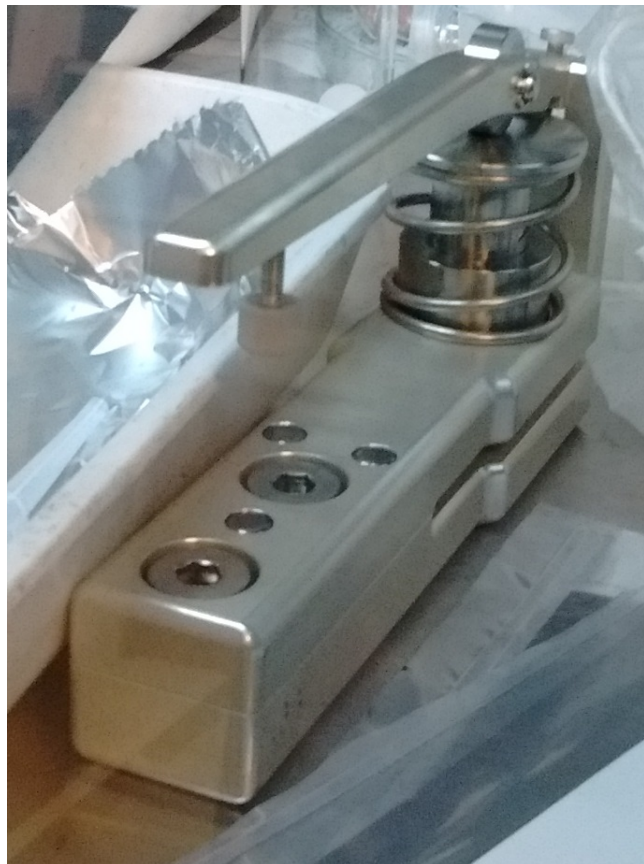
(a) Disk puncher used to make cell disks with a 15 mm diameter.
