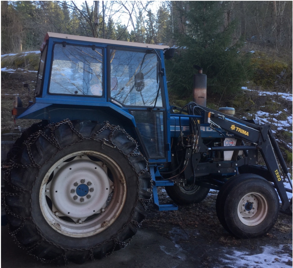
Picture 10: Nils showed me some of the equipment he uses in the production of field crops. Including this small, light tractor to avoid soil compaction.
