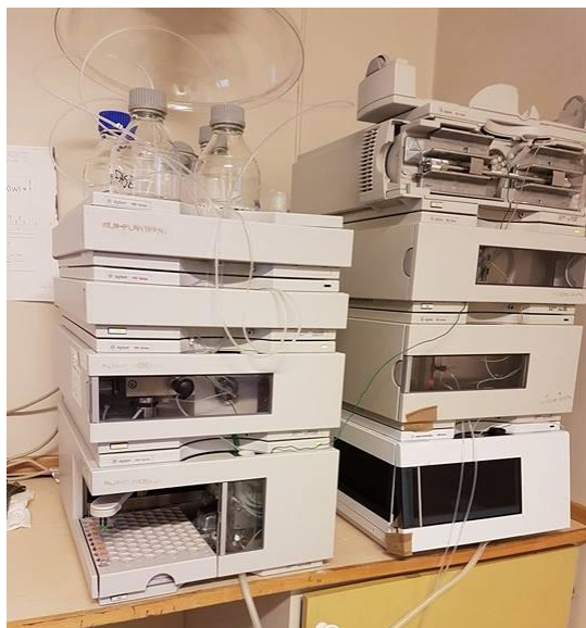
Figure 14. An Agilent 1100 Series HPLC system (Agilent Technologies, Waldbronn, Germany) equipped with an auto-sampler ( 4 \text{ }^\circ\text{C} ), a quaternary pump, an in-line degasser, a column heater and a photodiode array detector.
