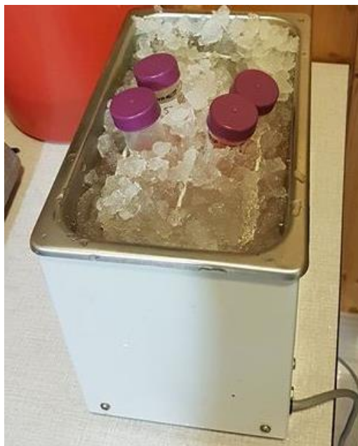
Figure 13. The samples in an ultrasonic bath (Bandelin SONOREX RK 100, Bandelin Electronic GmbH & Co., Berlin, Germany)
