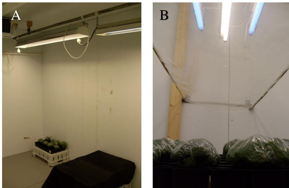
Figure 3.1.2. Visible light (A) and a combination of visible light with UV-B irradiation (B) treatments of broccoli during storage.
