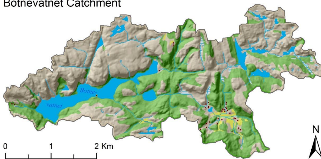
Figure 3. The delineated catchment for the lake Botnevatnet, including the accumulation raster with threshold=500, vegetation, land use and buildings. Data from The Norwegian Mapping Authority (DEM; N50) and NVE (Norwegian Lake Database).
