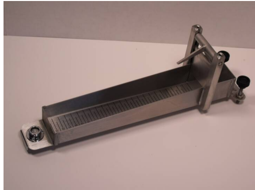
Figur 15: Bostwick consistometer (CSC Scientific Company Inc., VA, USA).
