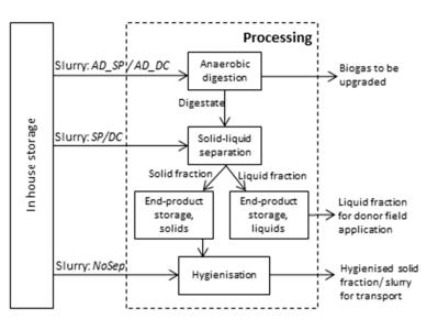
**Figure 3.** An overview of the processes included in the main process of "Processing" in Figure 2, indicated by the dotted line. The figure shows the processes (boxes) used under the different scenarios (in italics) to process slurry from in house storage and how the processes are connected by flows (arrows).
