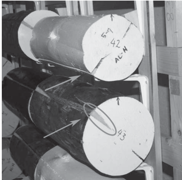
Figure 2. Specimens V-9 (42) and III-1 (43) in the rig. The water was sprayed from the left. The largest crack in each specimen was placed at a 45° angle on the horizontal plane, either upwards or downwards (arrows). The other crack was sealed with waterproof tape. Upward-facing cracks were sealed in each end of the specimen to prevent water from running out of the crack (ring).
