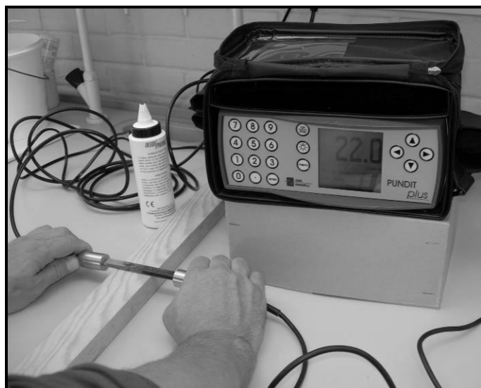
Figure 13. Pundit Plus, the ultrasound excitation device used in the experiments presented in Paper II. The transducers are pressed against the ends of the wood piece to be measured, and ultrasound waves are transmitted from one transducer and received by the other. The output from the device is transit time from one transducer to the other in \mu s.
