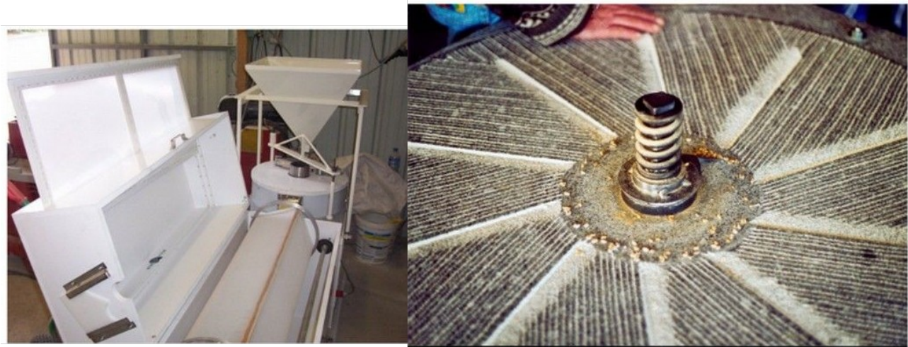
Figure 20: Astrié mill centrifugal reel (left) and millstone (right).
