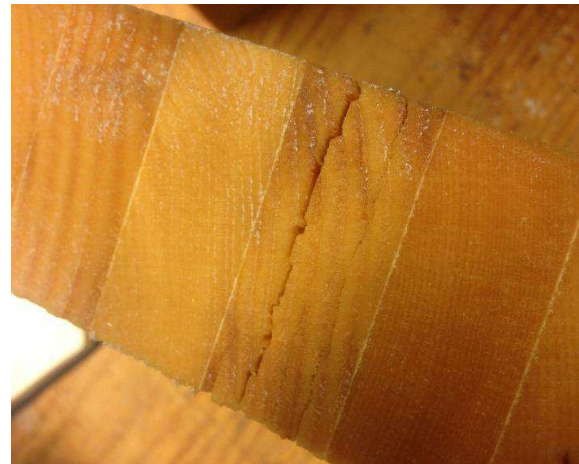
Figure 30: Splitting of the wood on the cross section of one of the samples after submersion in
