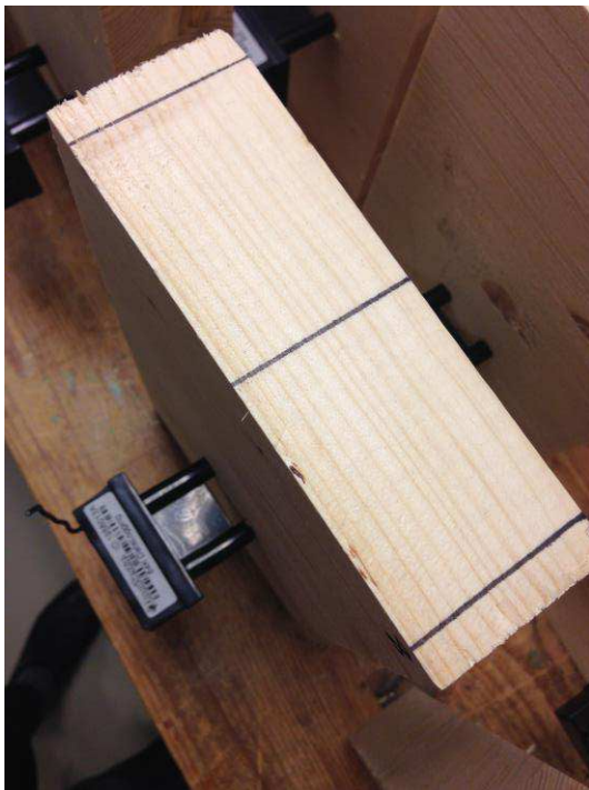
Figure 12a: One of the samples, with lines indicating where the height measurements are performed
