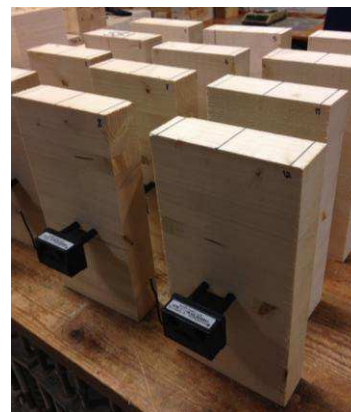
Figure 2: The twelve samples studied in the laboratory experiment, with sensors and measurement positions
