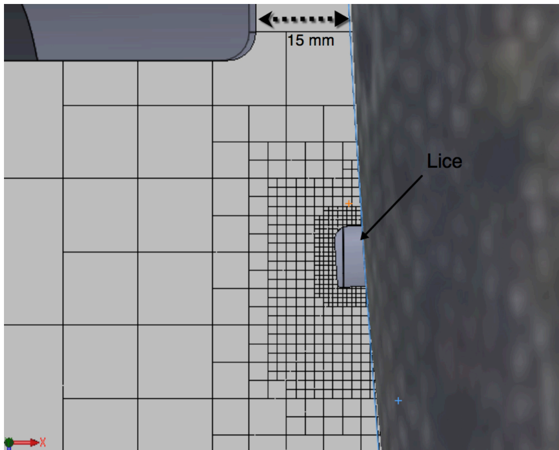
Figure 44: Cut plot of meshing. Initial mesh set to 4 and Local Mesh set to 6.
