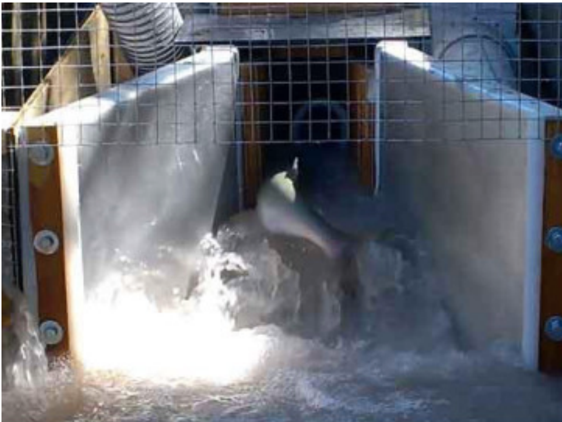
Figure 4: Showing the Fish Cannon attracting the salmon by using a waterfall.
