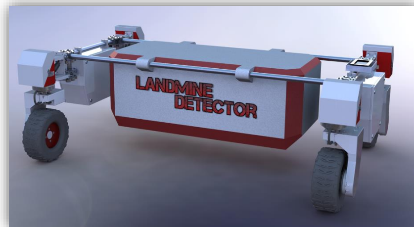
Figure 56: A possible solution for the robot, where only sensors are fitted to the robot.
