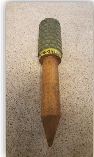
Figure 19: A PMR-2A AP fragmentation stake mine.
