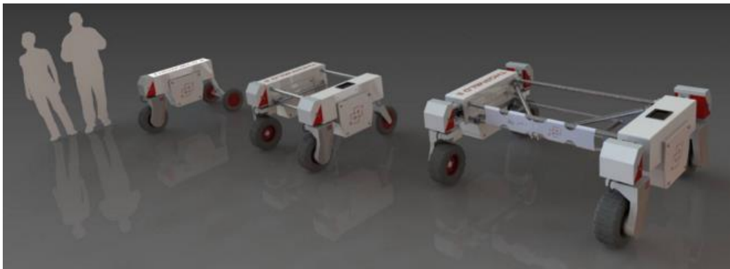
Figure 15: Thorvald 2 in three different models. From the left: One wheel drive and one wheel steering, two wheel drive (front) and two wheel steering (front), four wheel drive and four wheel steering. Courtesy of Lars Grimstad.
