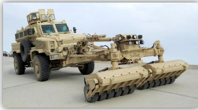
Figure 13: MMPV Type II (RG-31) with EHP Roller [20].
