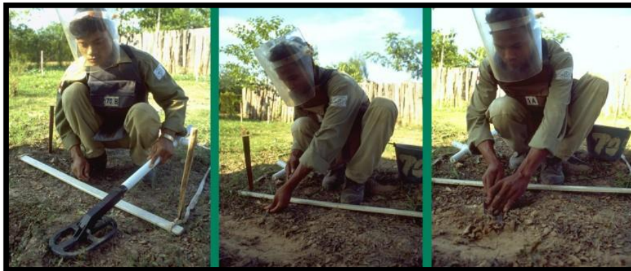
Figure 10: Manual demining method using metal detector and prodder [16].
