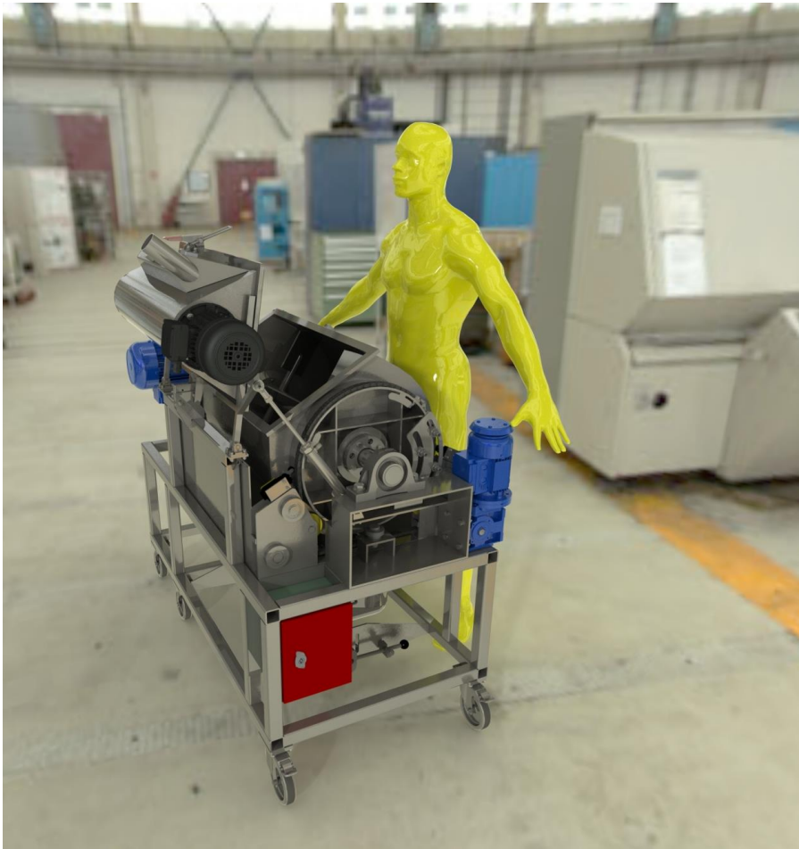
Figure 9.4: Mixer configuration in a production environment. Human (James) model provided by Sergio Skaletti (69)
