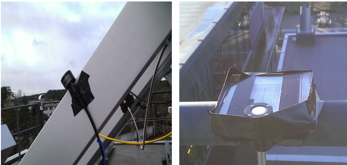
Figure 18: Diffuser tilted 37 degrees with respect to the horizontal (left) and diffuser positioned horizontally (right).
