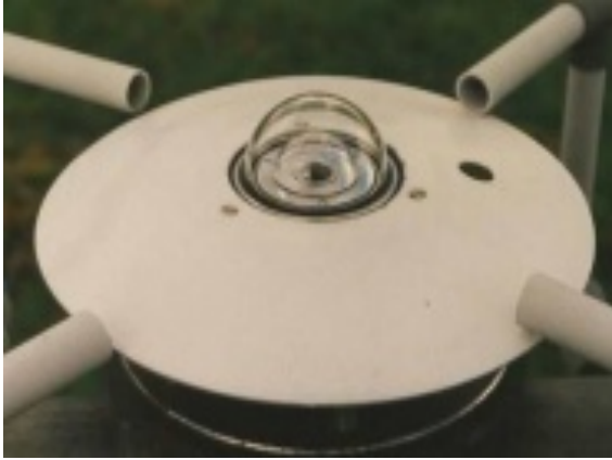
Figure 20: Eppley Precision Pyranometer used at the FAGKLIM site [39].
