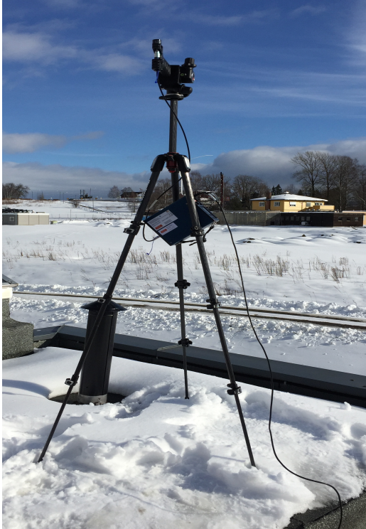
Figure 16: The measurement setup at Kjeller (left) and the diffuser-probe-connection (right). The diffuser is fastened to the probe with the black screw located on the left side of the probe.
