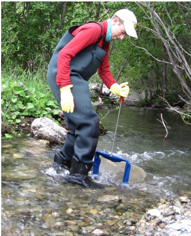
Figure 3. Photograph of the kick-sampler in action.
