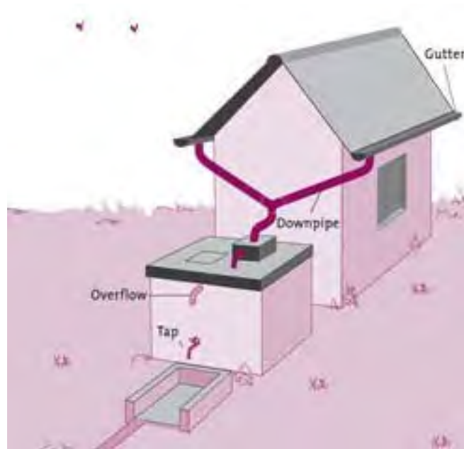
Fig. 1 Rooftop rainwater collection system (Smet 2003)
