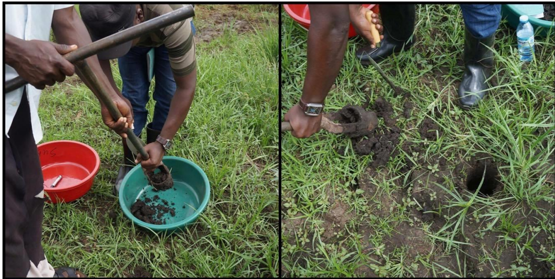
Figure 11 Image of soil sample collection using an auger during fieldwork (image taken by author)
