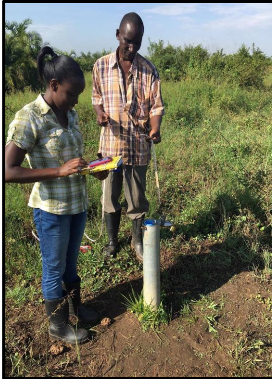
Figure 9 Slug test analysis on borehole 2 during fieldwork. (image taken by author)
