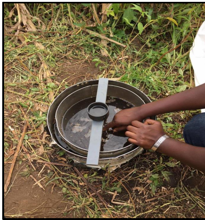
Figure 10 Double ring infiltration test conducted on the Eastern side of the aquifer during fieldwork (image taken by author)
