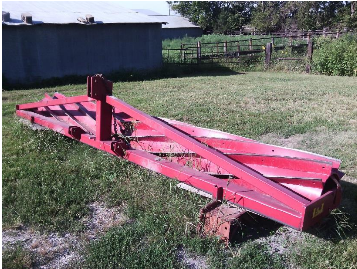
Figure 5: A roller-crimper, photographed on a conventional farm using no-till with cover crops.
