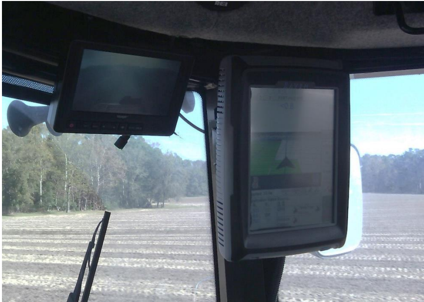
Figure 4: Precision equipment applying variable-rate fertilizer.
