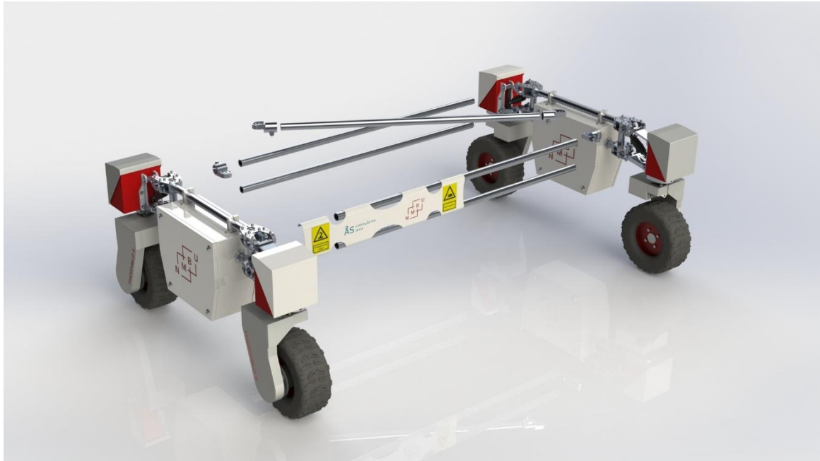
Figure 5-47. The robot are divided into two nacelles connected by a frame.
