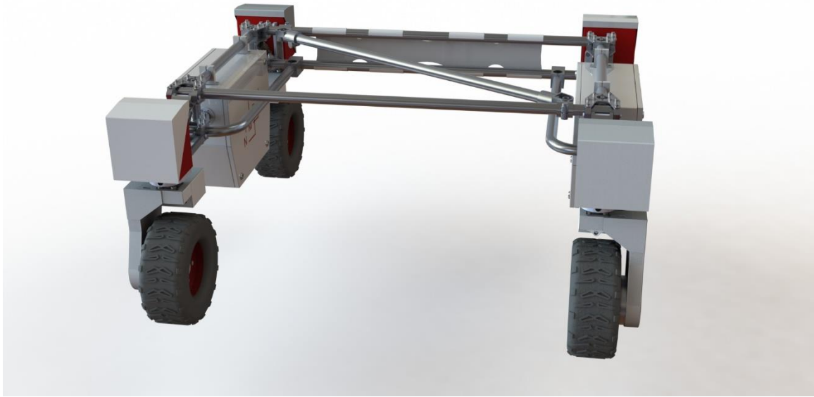
Figure 5-23. Using rails on the lower frame, the tool can be centered onto the rails with the help of the bended rail ends shown on the rendering.
