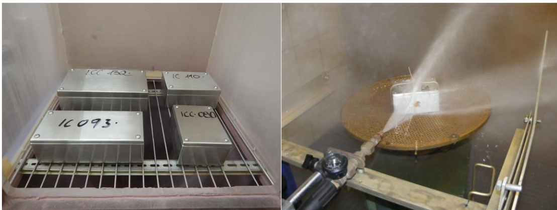
Figure 8-1. These pictures show us examples on IP-grading tests conducted by the TZO/LUW laboratory in Germany. Picture to the left shows enclosures tested in a dust cabinet, while the picture to the right shows how the enclosures tested against high-pressure water jets [52].
