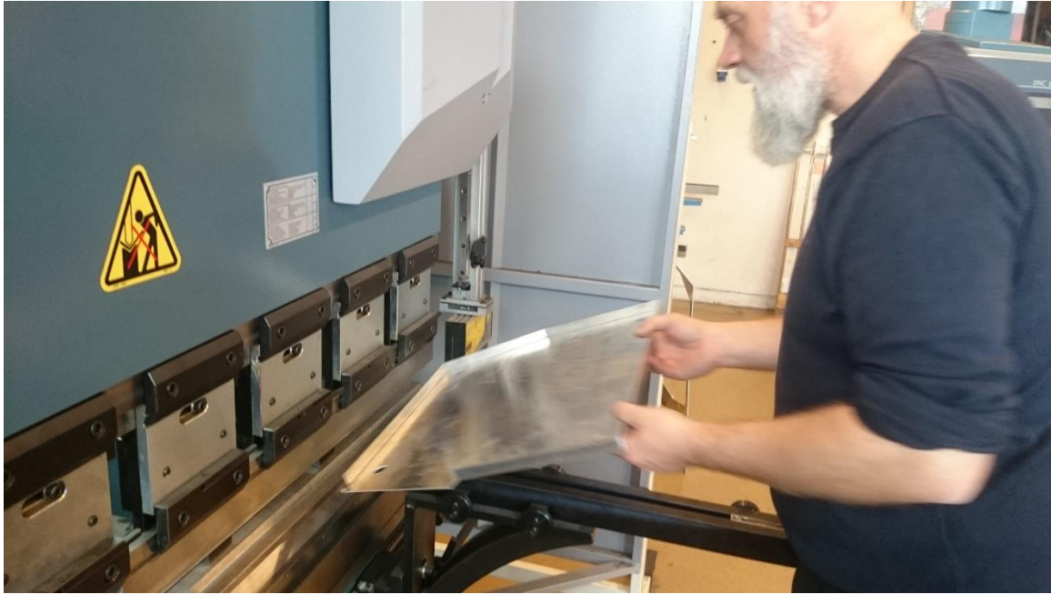
Figure 6-3. A photo of our helpful Rune Stensrud, teacher of production processes at Ås high school, here working with bending press forming machine, producing the lids of the electronic box...
