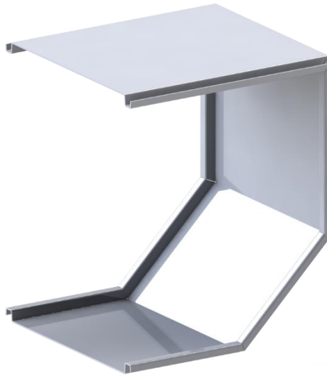
Figure 5-17. One of my very first ideas on how the electronic compartment should look like. Two of these halves were to be welded together, and a lid was placed on each side of the box. Note the double flange more closely described in Figure 5-18
