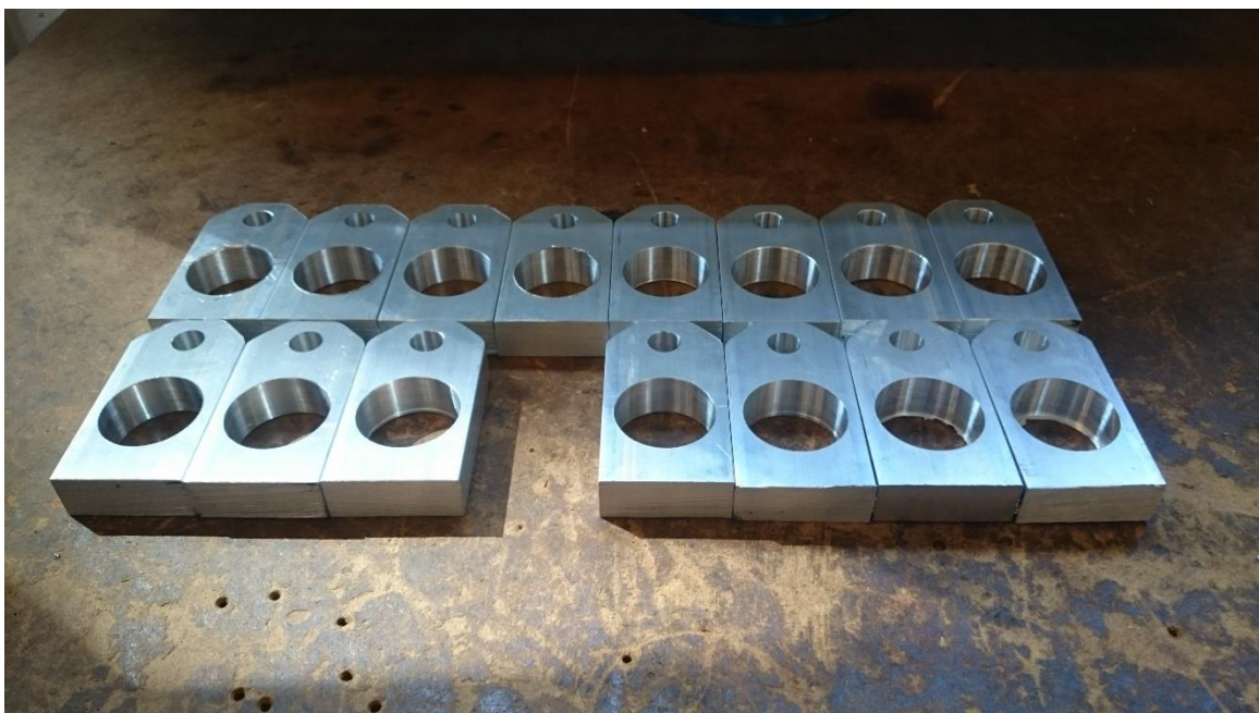
Figure 6-8. Hinge tube clamps nearly finished after CNC-milling.
