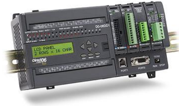
Figure 9-17. Image shows an example of a programmable logic controller by DirectLOGIC [77].
