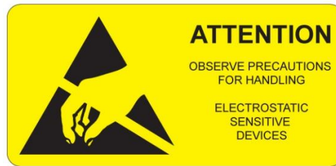
Figure 9-27. If a symbol like this is present on electronic components, show extreme caution to not destroy the object [90].
