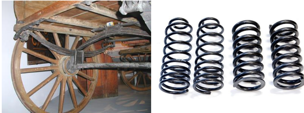
Figure 2-8. Leaf springs have been used since the 1800s, while helical compression springs is the most used in the automotive industry today [21] [22].
