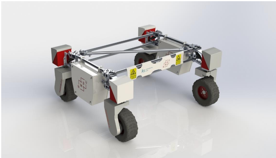
Figure 5-46. Fully assembled robot with visible frame, without covers.
