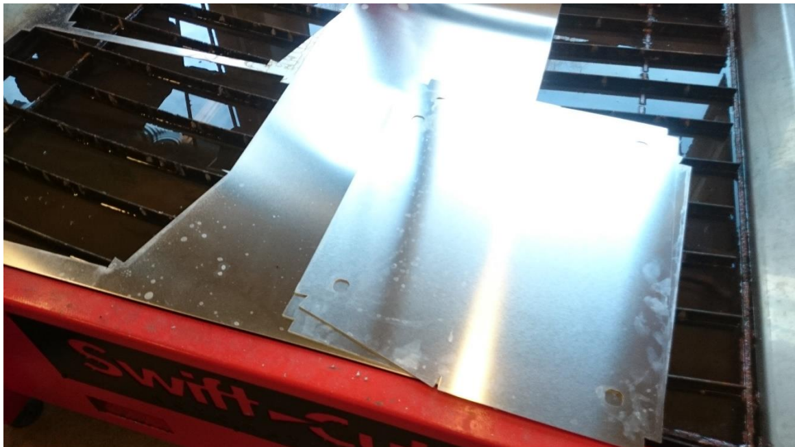
Figure 6-2. Lids for the electronic compartments after being plasma cut.
