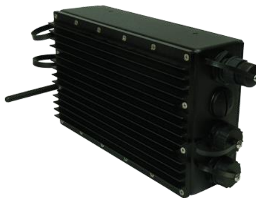
Figure 9-1. The SmallPC iBrick 215ML featured with waterproof IP67 enclosure [55].
