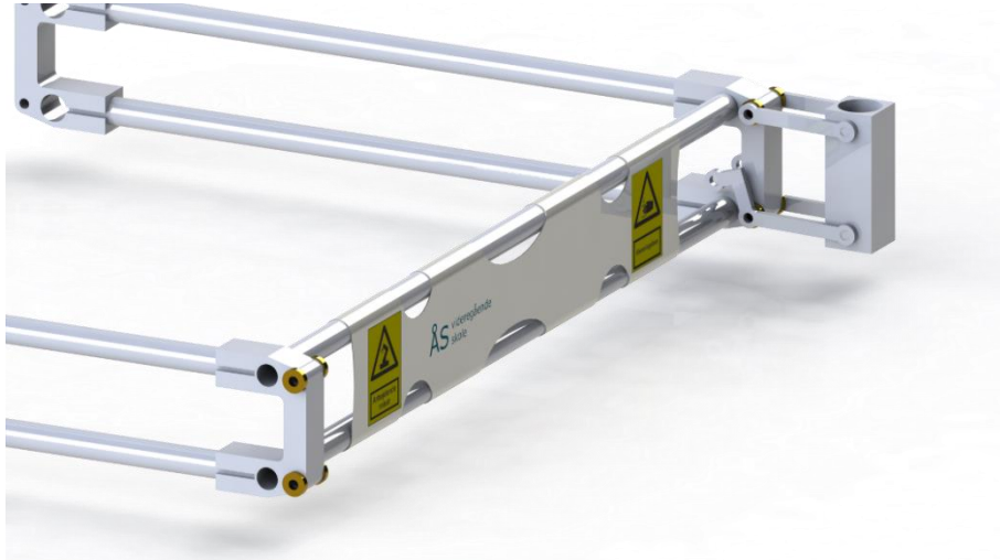
Figure 5-4. One of the first ideas of tube connection design and suspension. This required a lot of aluminum material and a lot of machining hours.
