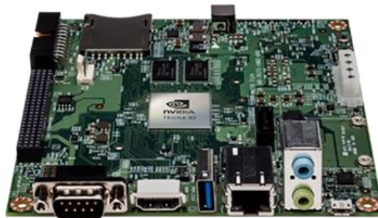
Figure 9-3. Illustration of the small and lightweight NVidia Jetson TK1 Embedded Development Kit [59].
