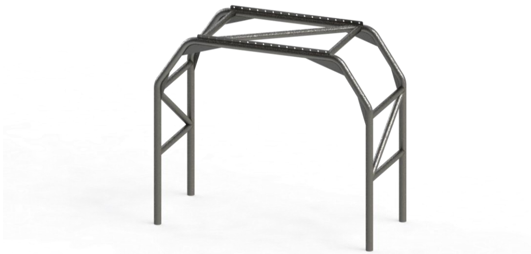
Figure 5-11. Using pre-fabricated roll cage hoops, it is possible to weld together simple elements and the required stiffeners to gain the desired stiffness.
