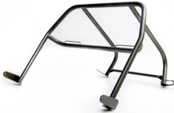
Figure 5-10. This illustration shows us a typical roll cage for cars, complexity varies with cars. Image Courtesy of
