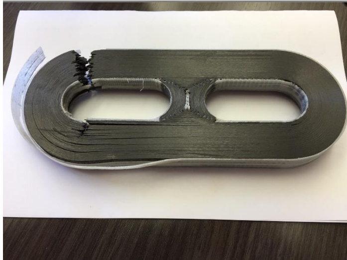
Figure 4-1. Using a composite 3D printer, a blog claims that this printed chain link required a 10 tonn weight to break.
