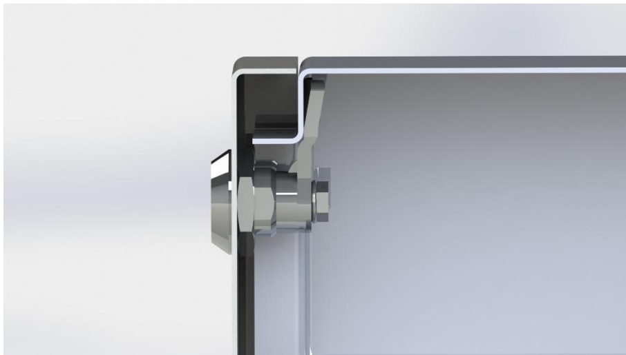
Figure 5-22. Cross section of the final solution of an aluminum enclosure and locking mechanism from KIPP. Notice the spacing between the lid and the lip for rubber seal fitting.
