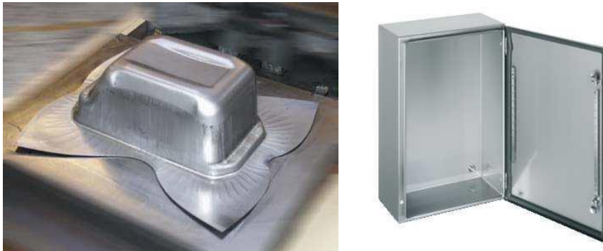
Figure 4-2. This image shows a deep drawn metal container, and a sheet metal enclosure produced by bending. [38] [40].
