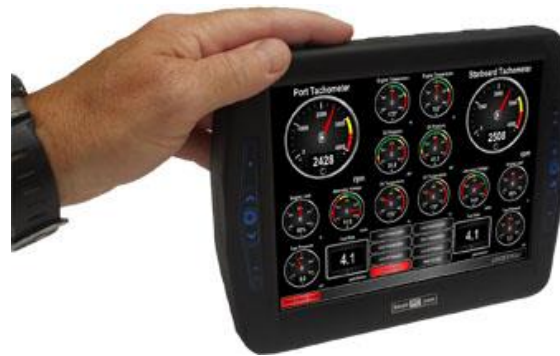
Figure 9-10. The SunVU RWD085M. A high brightness IP65 freestanding, clamp-able screen. An idea is to clamp this screen to the tube frame. Easy to take off when job is done [66].
