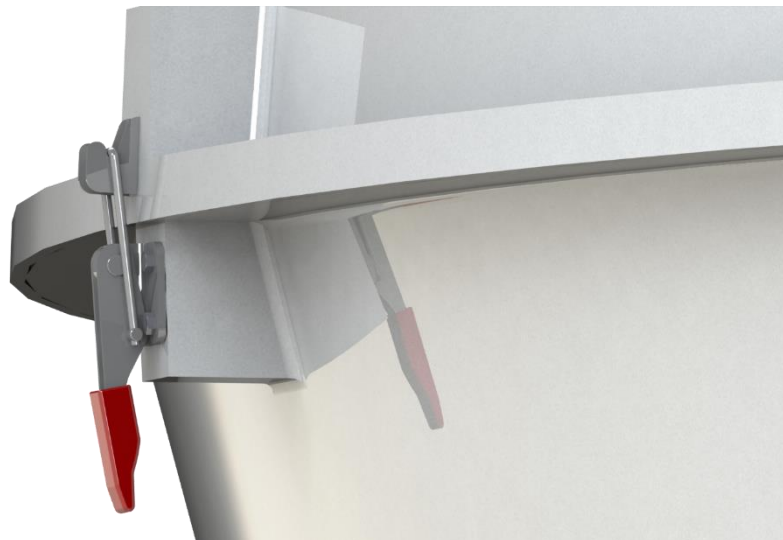
Figure 5-20. The idea for the composite enclosure involved latches and a compression flange containing a gasket.
