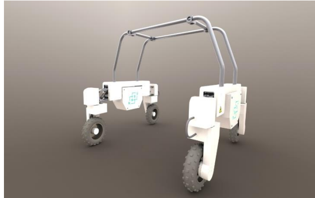
Figure 5-9. Thora extension by using two single tubes bended into a double hoop structure.
