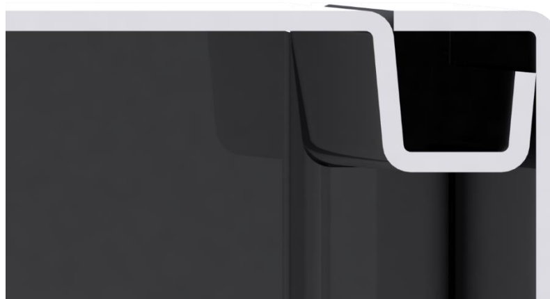
Figure 5-18. Double flange can in combination with a rubber seal create a reliable seal by deflecting water jets and avoiding straws of grain being wedged into the seal.
