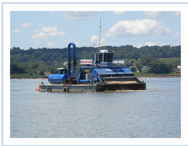
Figure 4. Hydraulic spreading application unit at Onondaga Lake, Syracuse, NY.
