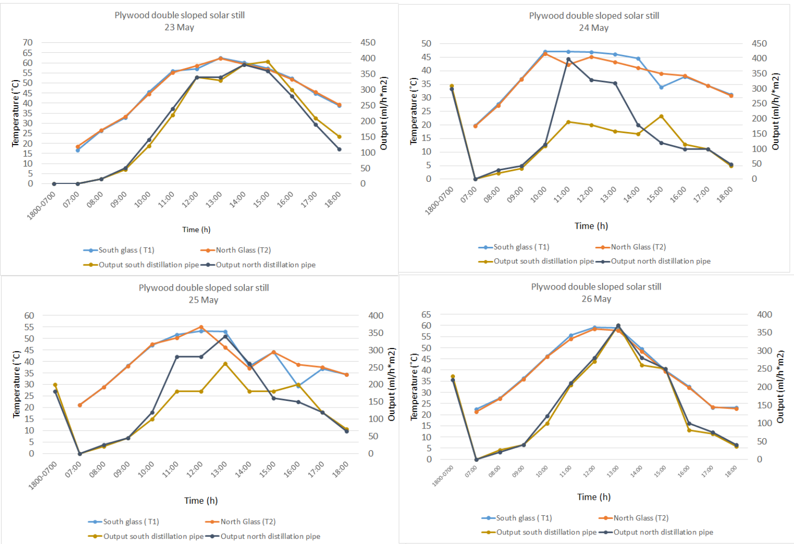
Figure 18: Showing the effect on the glass temperature when performing outside cooling by a wet blanket, on the 24 th and 25 th of May. 23 rd and 26 th is days with normal conditions. Real output (ml/m 2 ) in is shown for the north and south distillation channel.
