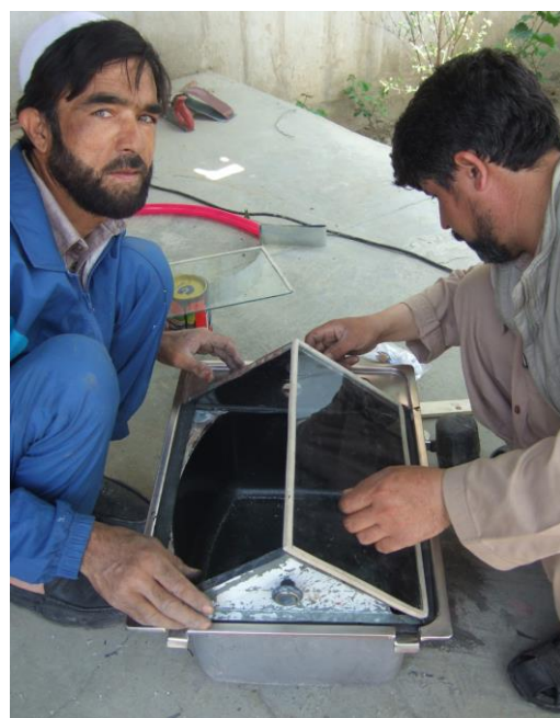
PICTURE 12: CARPENTERS INSTALLING THE GLASS COVER ON THE SINK DOUBLE SLOPED SOLAR STILL
