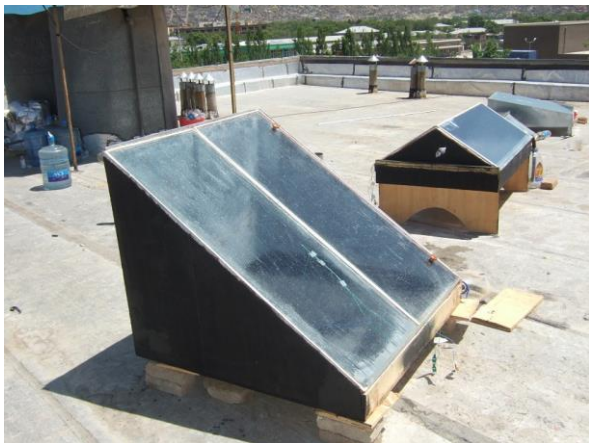
PICTURE 3: THE PLYWOOD SINGLE SLOPED AND THE PLYWOOD DOUBLE SLOPED SOLAR STILL
