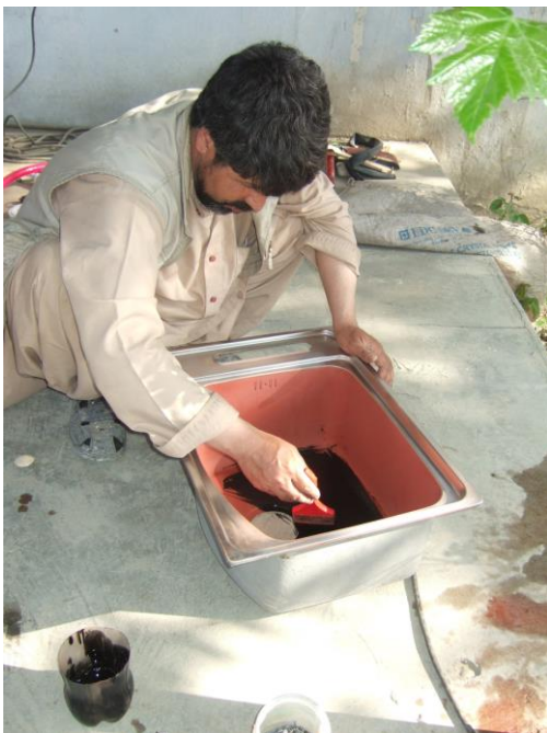
PICTURE 9: PAINTING THE BASIN OF THE SINK DOUBLE SLOPED SOLAR STILL
