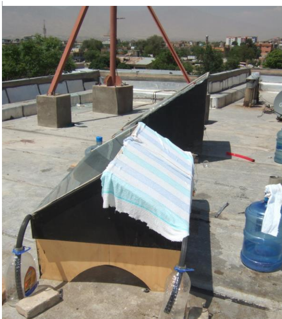
PICTURE 5: COOLING OF THE GLASS COVER BY AT WET BLANKET ON THE PLYWOOD DOUBLE SLOPED SOLAR STILL.
