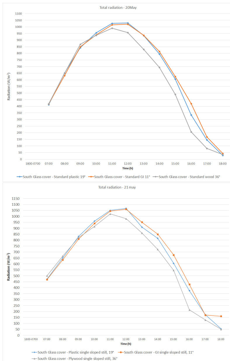
Figure 34: : Received radiation in W/m^2 on the glass cover of the GI single sloped solar still ( 11^\circ ), Plywood single sloped solar still ( 36^\circ ), and Plastic single sloped solar still ( 19^\circ ), on the 20 th and 21 st of May.
