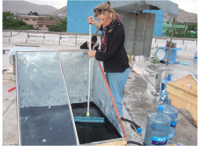
PICTURE 14: MAINTENANCE ON THE PLYWOOD SINGLE SLOPED SOLAR STILL
