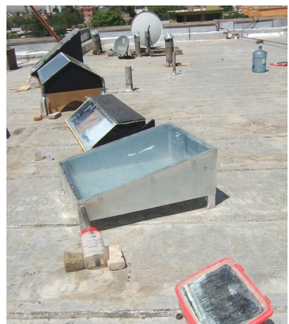
PICTURE 6: PLASTIC SINGLE SLOPED, GI SINGLE SLOPED, WICK STILL, PLYWOOD DOUBLE SLOPED AND PLYWOOD SINGLE SLOPED SOLAR STILL
