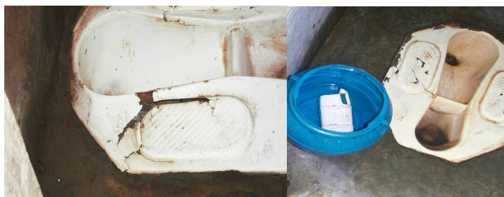
Figure 14: (photo: Kaia Bing) example of crashed up pan and broken pan from one of the interviewed households.
