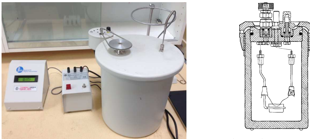
Figure 5-7: Parr® Oxygen Bomb Setup (Left) and Drawing of Internal Components of Oxygen Bomb
