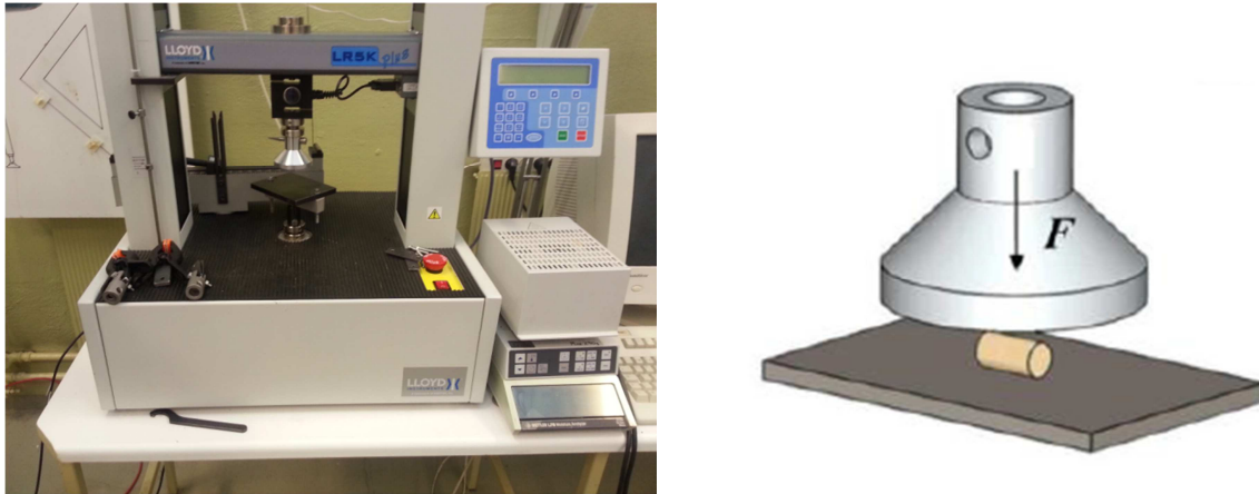
Figure 5-6: Lloyd LR5K (Left), and Diametral tests of feed pellets* (Right) *Diagram from Salas-Bringas et al [11]
