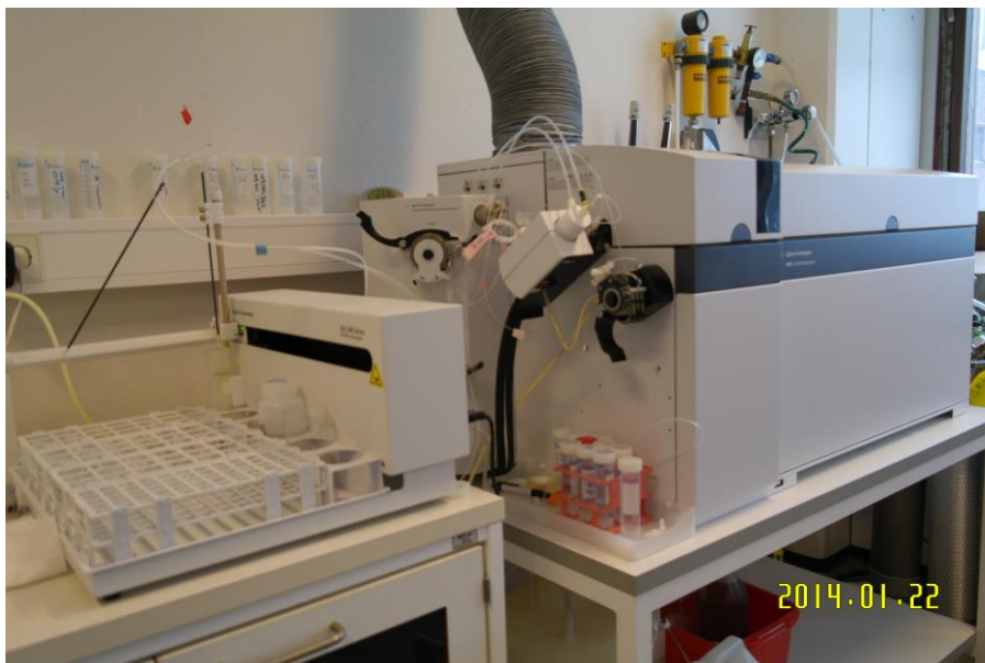
Figure 14: Triple quadrupole inductively coupled plasma-mass spectrometer model 8000 equipped with automatic sampler from Agilent, USA
