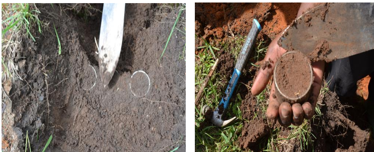
Figure 6: Soil sampling for bulk density analysis based on core method
