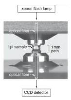
Figure 15: Nanodrop measures nucleic acids concentrations between two optical fibers using light from a xenon flash lamp detected by spectrometer. Picture obtained from: <u>http://nanodrop.com/Library/CPMB-1st.pdf</u>.
