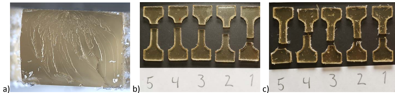
Figure 84. Image of the rupture of a T2-39-specimen. b) The dog bone specimens of T2-39. c) the dog bones specimens of T2-40.
