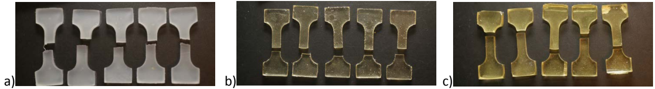
Figure 36. Sample specimens subjected to tensile testing. a) EP1900/N100 (T2-6) b) GAP/N100 (T2-7) c) HTPB/IPDI (T2-8)
