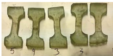
Figure 95. Dog bone samples of T3-5 (GAP/N100/TMETN/PEG).
