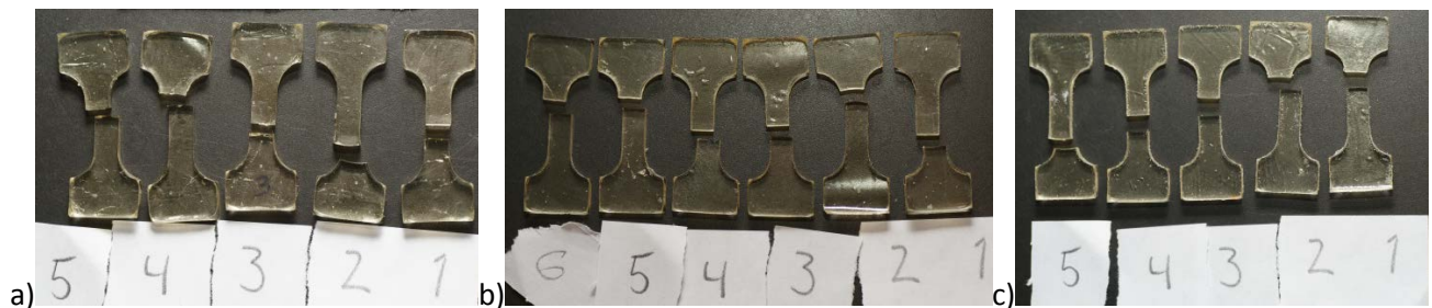
Figure 45. Dog bone samples subjected tensile testing, GAP/IPDI/N100 samples with an NCO:OH ratio of a)1.0 (T2-29) b)1.2 (T2-30) c) 1.4 (T2-31).
