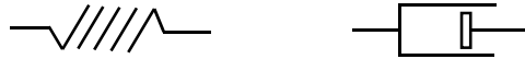
Figure 19. Left: elasticity explained by a spring, energy is stored. Right: dash pot, applied energy dissipates. In a viscoelastic polymer, both of the properties are represented.
