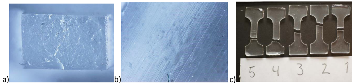
Figure 58. images of tensile tested dog bone specimens of T2-42. a) b) one can observe some phase separation close to the bottom-faced surface of T2-42. c) the dog bone specimens of T2-42.
