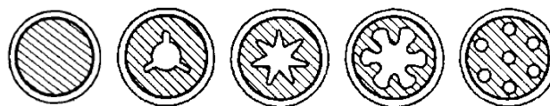
Figure 6. Cross-sections of different propellant configurations. From the left: End-burner (neutral burn), slots and tube (neutral), star (neutral), wagon-wheel (neutral), Multiperforated (progressive-regressive). Objects are exported from (Sutton and Biblarz 2001).
