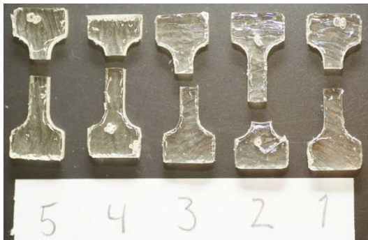
Figure 165. tensile tested specimens of sample T2-41. A rough surface, but surprisingly precise tensile results. Voids were apparent, but effectively avoided.
