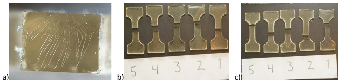
Figure 88. images of broken dog bones a) the broken surface of T2-44. b) tensile tested dog bones of T2-44 c) T2-45.
