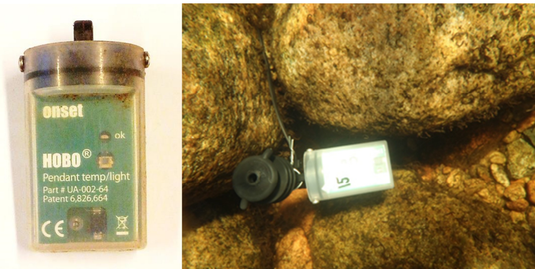
Figure 19. HOBO® logger for measuring temperature and light time series in Kvina (Station 1, 2, 4 and 5).
