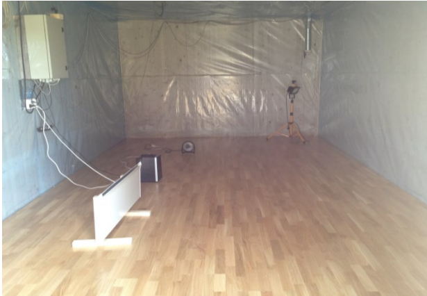
Figure 2: Interior view of module B where the walls and ceiling are upholstered in PE foil.
