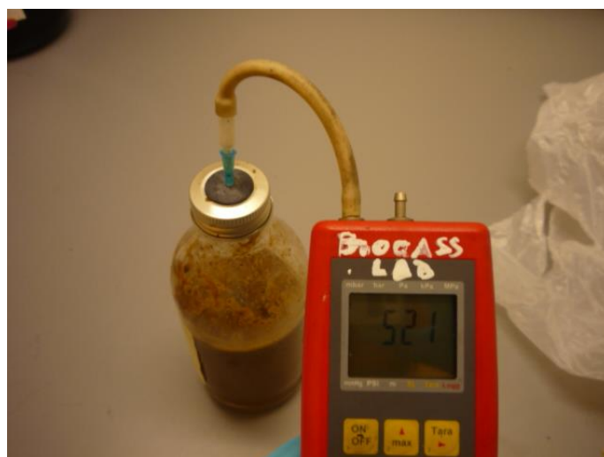
Figure 5.2. Gas pressure measurement with electronic pressure gauge. Photo: I. Georgiadis (2013).
