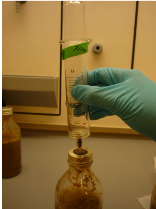
Figure 5.3. Gas volume measurement with 50 ml glass syringe. Photo: I. Georgiadis (2013).
