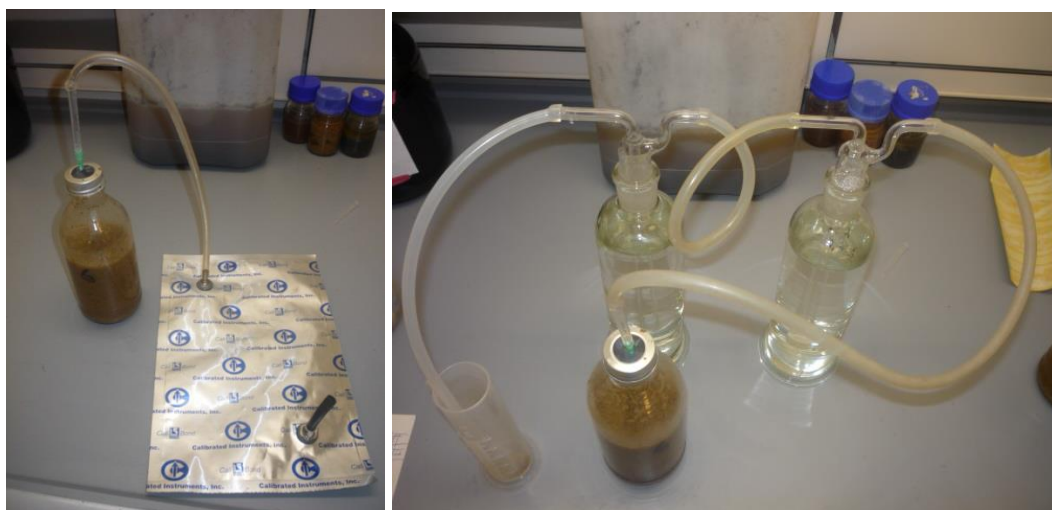
Figure 5.4. Alternate methods of gas measurement. Photos: I. Georgiadis (2013).
