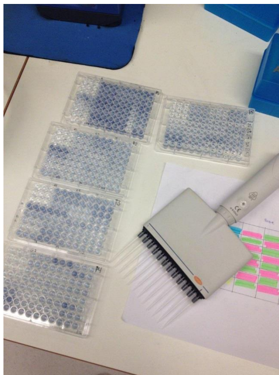
Figure 14. Analysis of protein concentration in tadpole cytosol prior to the glutathione S-Transferase (GST) assay. Photo: Eivind Farnen.
