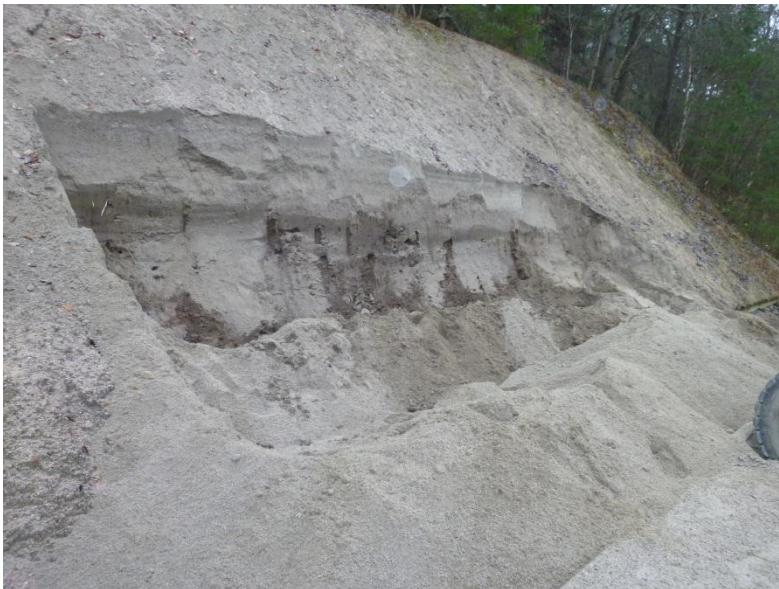
Figure 5. Soil profile with a clear view of homogeneity of the soil. (Photo: Liland, 2012)
