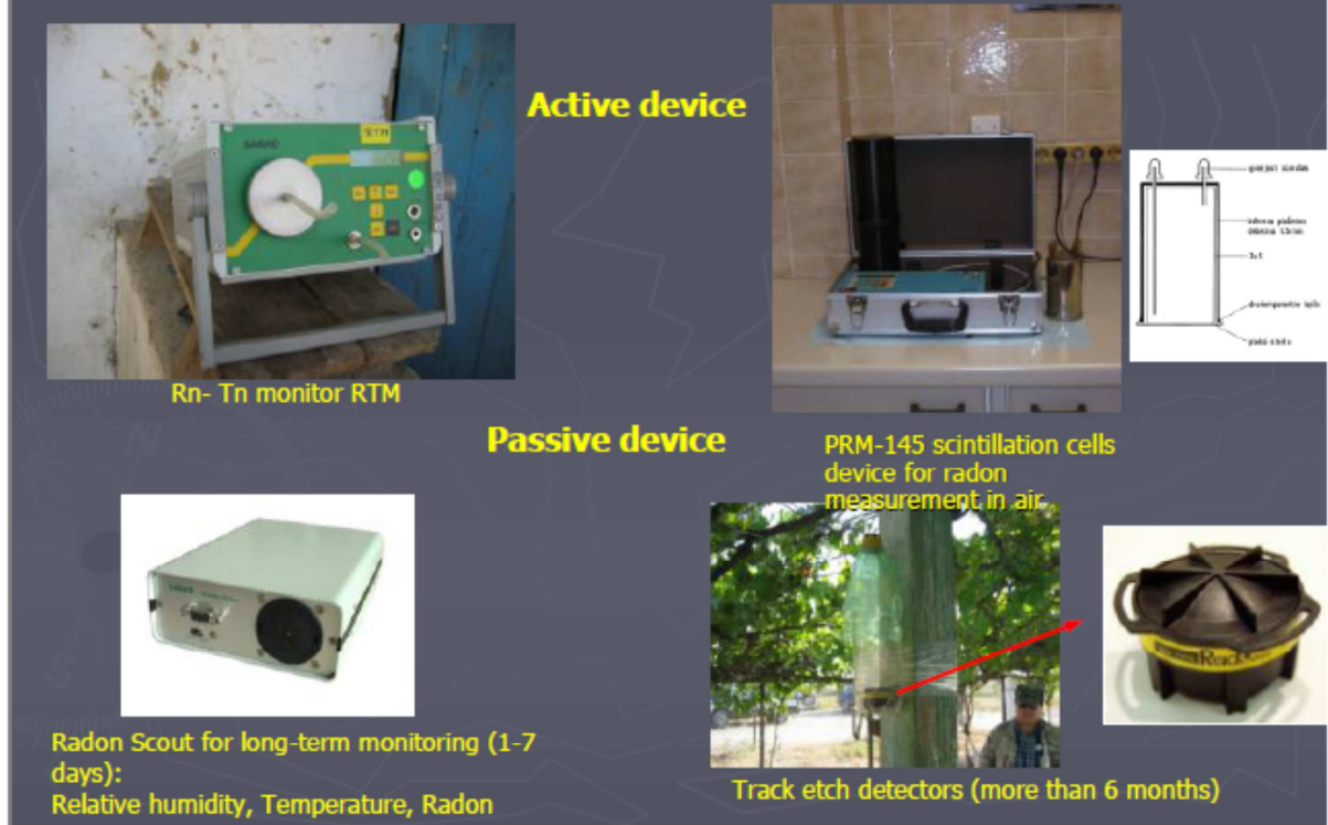
Figure 10: Active and passive devices used for instantaneous Rn measurements and SSNTDs used for long term Rn measurements (Salbu et al. 2011).
