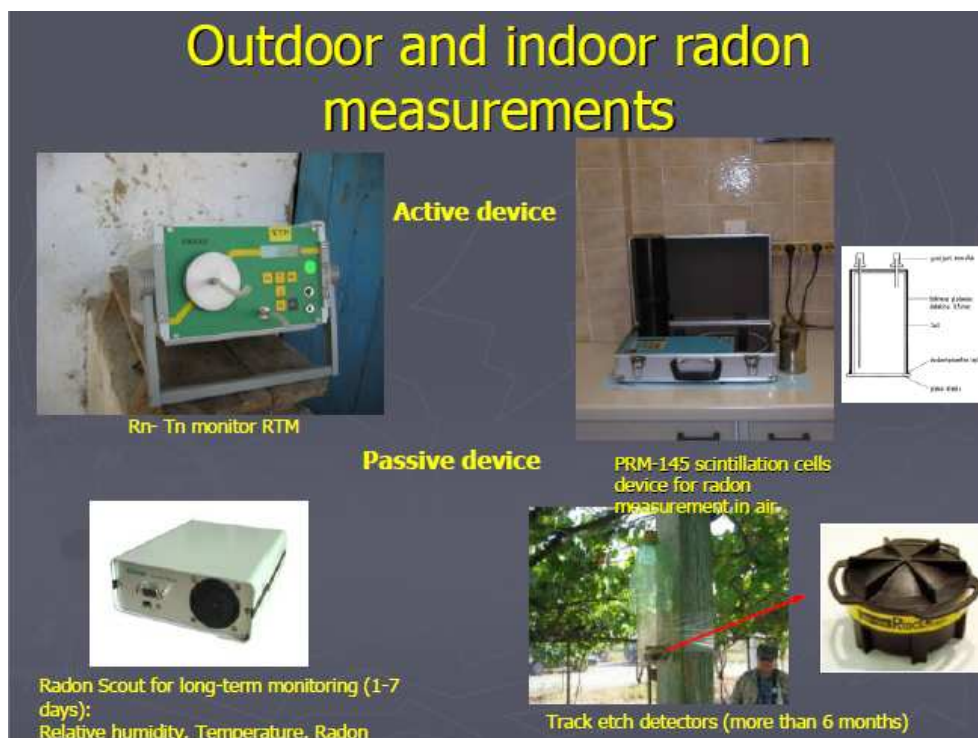
Figure 10. Active and passive radon measurement devices (Salbu et al. 2011)
