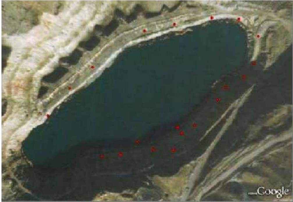
Figure 10. Gamma dose rates measured along the pit lake (Salbu et al. 2011)
