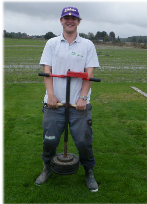
Figure 17: The apparatus was dropped from 10cm at each plot. Photo: Trygve Aamlid
