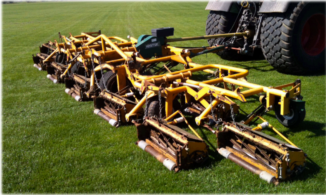
Figure 11: Kesmac 11 gang cylinder mower. photo: http://www.vanmac.nl
