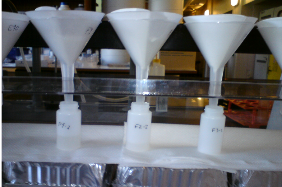
Figure 4: The setup used in sequential extraction; a funnel holder, funnels, filters and sample vials.
