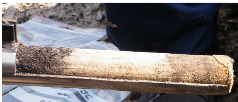
Figure 3: Corer with front panel pushed back and revealing a soil sample. This specific sample was from site 3, 2010. The burned top soil is visible.
