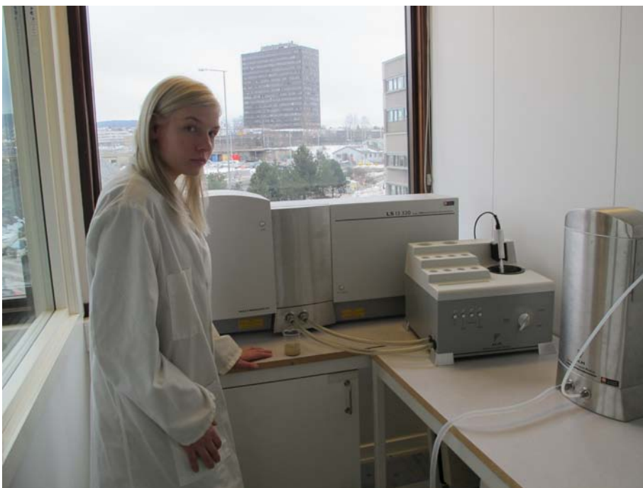
Fig. 11: Grain size distribution analysis with the Coulter laser diffraction particle size analyser
