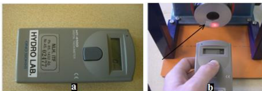
Figure 14.4. a.) The tachometer. b.) A white sticker is attached to the turbines axel (shown via black arrow). The tachometer is aimed and held stationary at a point where the sticker passes. One needs to hold the tachometer steady at this point for longer than five seconds in order to receive accurate readings.
