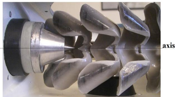
Figure 13.7. The centre of each blade was checked to line up with the water nozzles tip. None of the blades were perfect but most were very close. The nozzles axis from its tip has been drawn over the picture as a black line. Here the entire axel had to be nudged upwards for the blades to align better.
