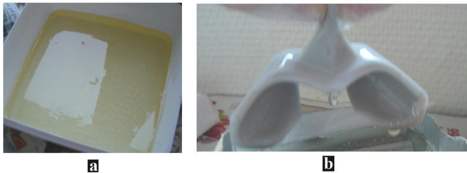
Figure 13.5. a.) The epoxy bath used to soak the blades in. b.) After 10 min, the blades stop producing bubbles and are removed for drying.
