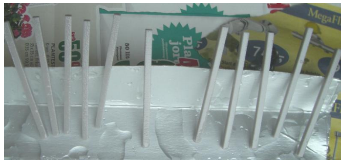
Figure 22.2. The test rods. Each rod had a square cross-section of 3 \times 3 \text{ mm} and was 45 \text{ mm} long. Drying took 2 days at room temperature.
