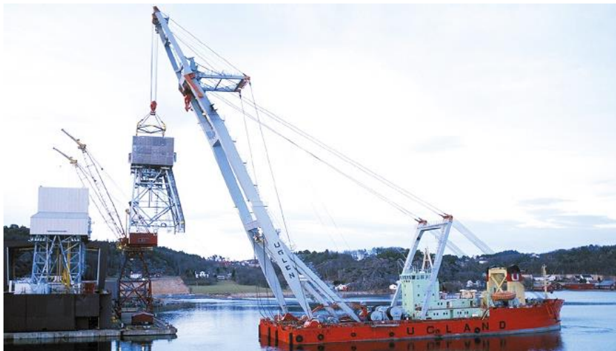
Figure 38: The self-propelled heavy lift crane vessel HLV Uglen (Ugland Construction AS 2013)
