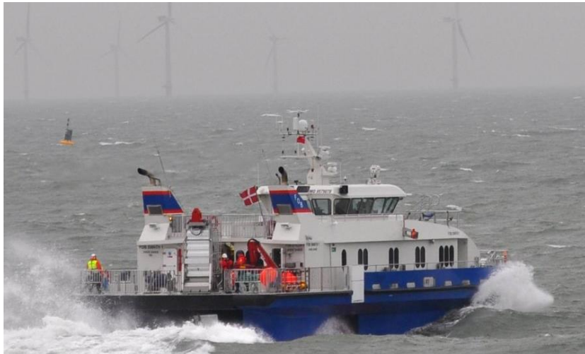
Figure 85: Maintenance operation with the FOB SWATH 1 at Greater Gabbard (Odfjell Wind AS 2012)
