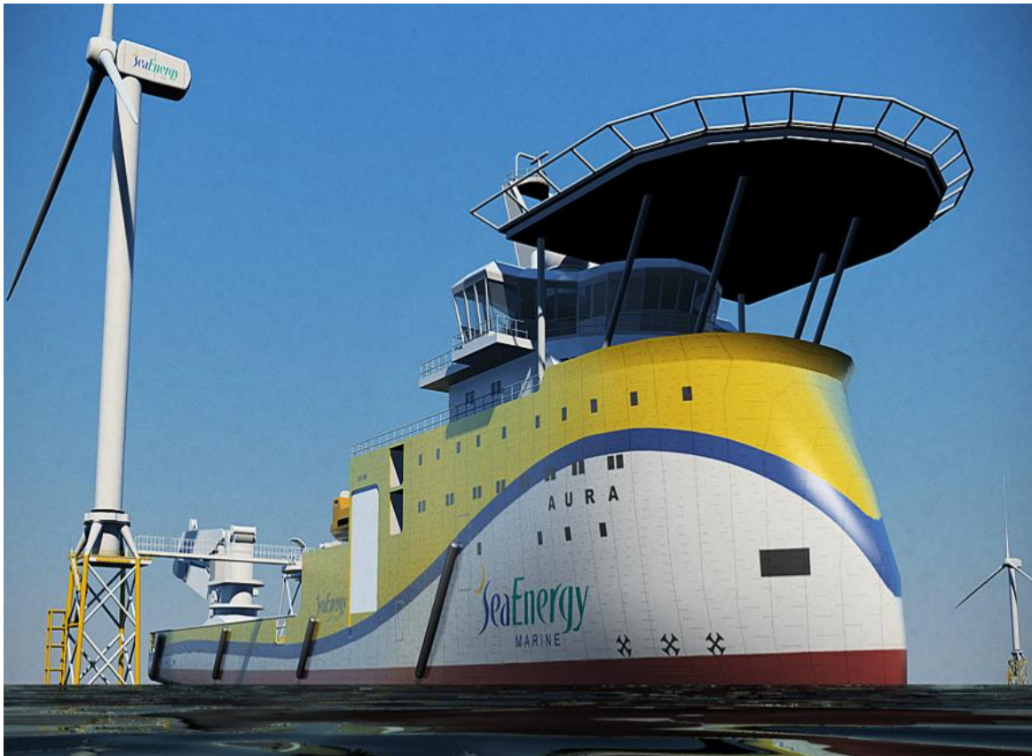
Figure 42: Illustration of an offshore mother vessel developed by Ulstein and SeaEnergy (SeaEnergy PLC 2012)
