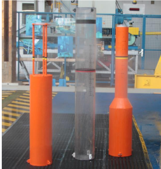
Figure 22: Models tested in wave tank. From left to right; TLB X3, Simple reference model, TLB B
