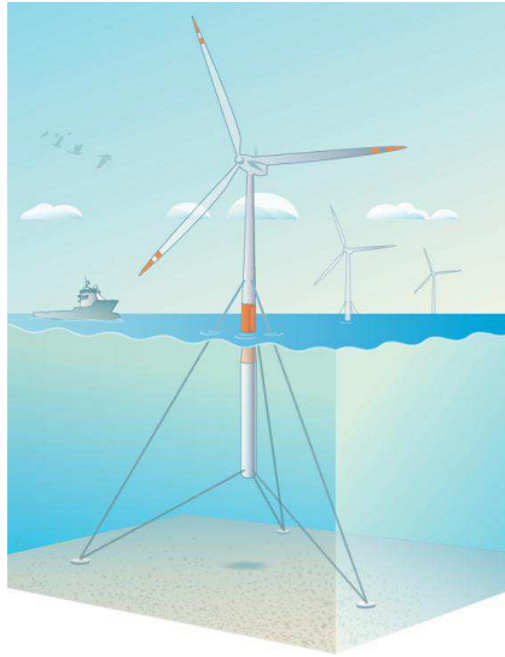
Figure 5: The TLB Concept (Myhr & Nygaard, Load Reductions and optimizations on a tension legged buoy offshore wind turbine platforms., 2012)
