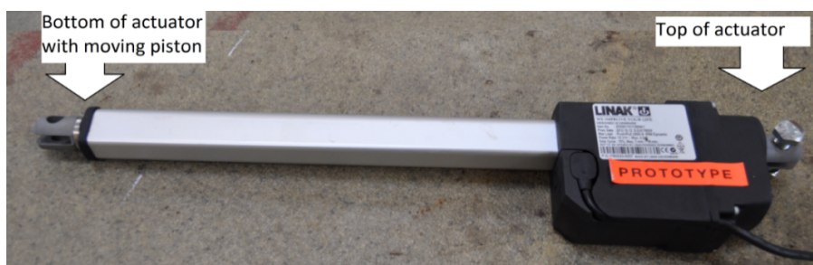
Figure 31: Linear actuator LA23 from LINAK
