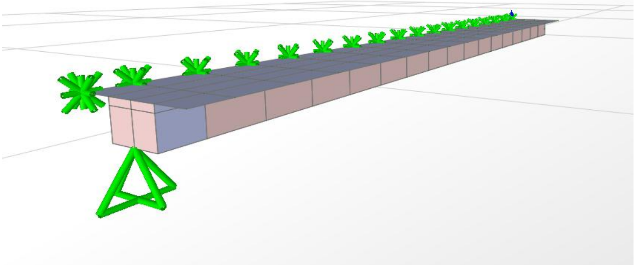
Figure 2: Shell model in 3D from SAP2000.
