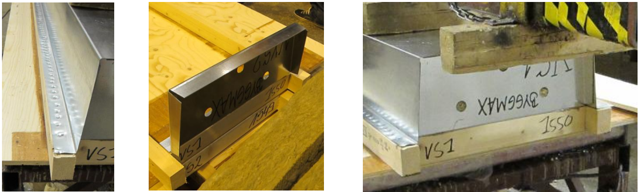
Figure 2a (left): Upper steel flange and wood row. Figure 2b (middle): Support plate. Figure 2c (right): Support plate with wood ribbon mounted on metal sheeting. (Pictures are taken when the elements are mounted upside down in fabric.
