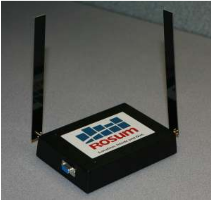
Figure 5-9, the Rosum User Device with dual antennas
