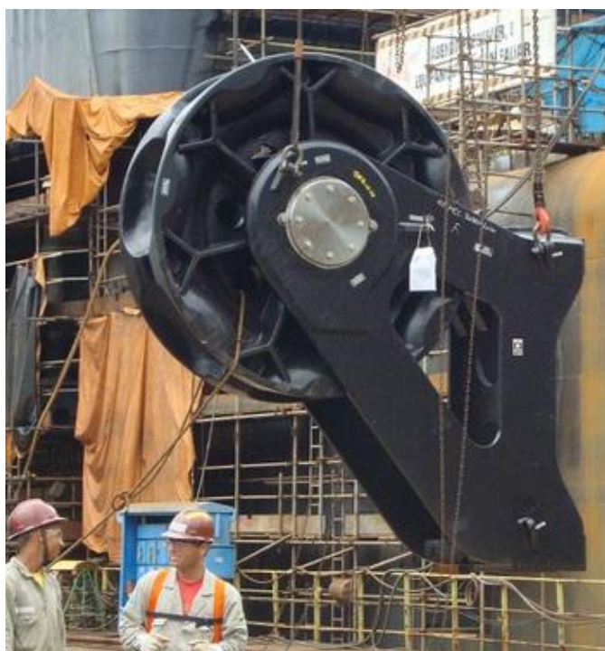
Figur 43 - Fairled for montering under vann (Timberland Equipment Limited, 2011).
